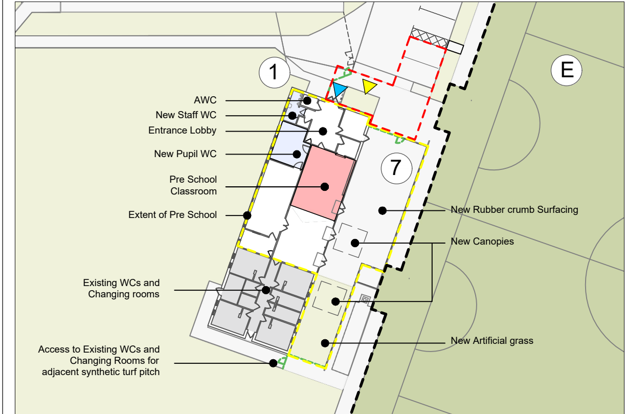
Refurbished Pavilion Building 0 5 10 15 20 25m 1:500 @ A3
